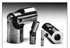
Boston Gear precision machined J and JS Series Universal Joints are designed for connecting shafts at angles up to 30 degrees and speeds up to 2000 RPM. All sizes are stocked with both solid and bored hubs.
